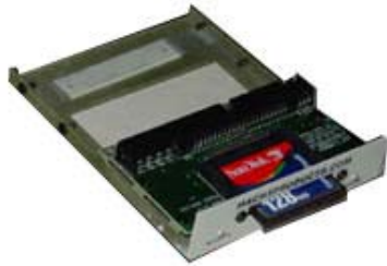
Adapter mounted in front position
