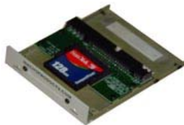
Adapter mounted in rear position
